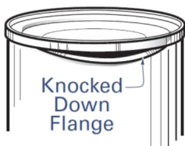
**Gambar 4.** Cacat *knocked down flange*
